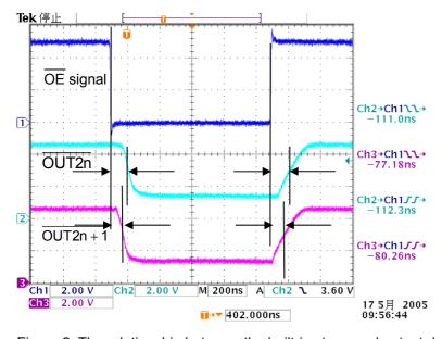
Figure 2. The relationship between the built-in staggered output delay and  $\overline{\text{OE}}$  signal
